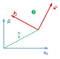
• Homogeneous Transformation is a convenient way to write the formula in a  $4\times 4$  matrix:
