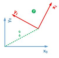
• Homogeneous Transformation is a convenient way to write the formula in a  $4\times 4$  matrix:
