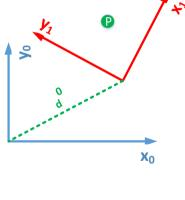
• To use HTs in computing coordinates of point *p*, we need to extend the vectors of a point by one coordinate:
